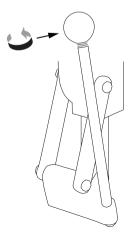
Tighten up strongly and apply thread-lock
